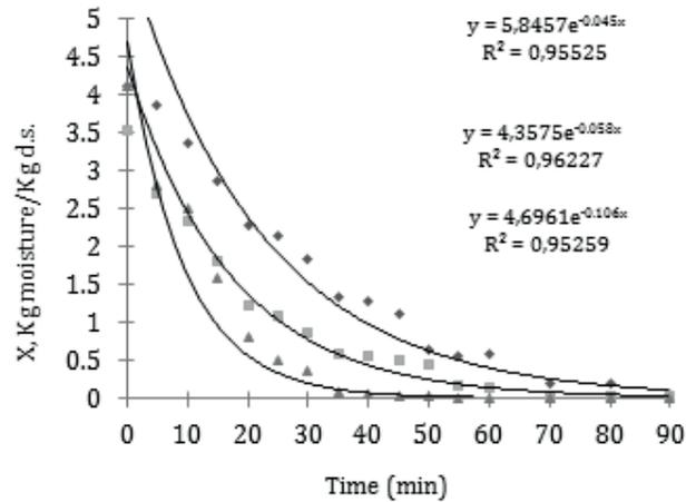
**Figure 1.** Drying kinetic performed for banana miniflakes diameter of 2 cm and antioxidant concentration of 0,5 % (w/w). (♦) 50, (■) 60 and (▲) 70 °C.
