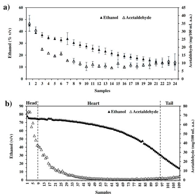
**Figure 1.** Behavior of ethanol and acetaldehyde during the first (a) and second (b) distillation of artisanal Mezcal. The vertical dotted lines on figure "b" indicate the distillate cuts. In figure "a", concentration values are given as the mean of the samples from two copper stills  $\pm$  standard deviation.
