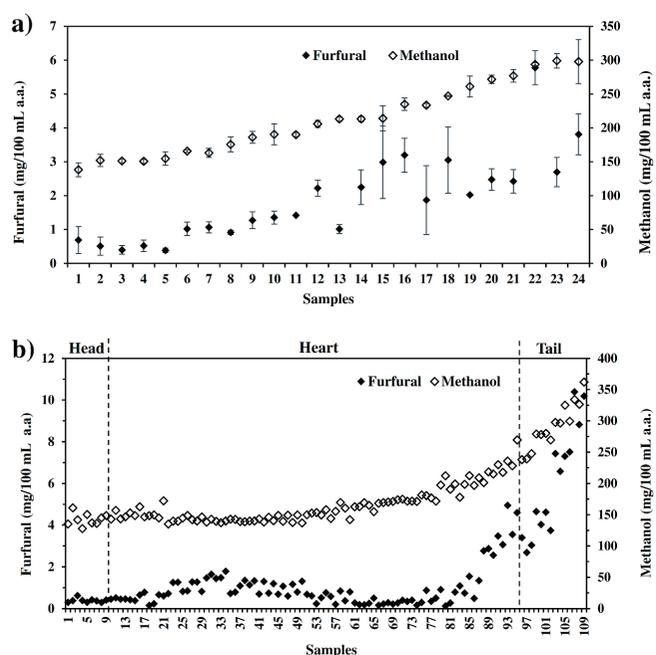
**Figure 3.** Behavior of methanol and furfural during the first (a) and second (b) distillation of artisanal Mezcal. The vertical dotted lines on figure "b" indicate the distillate cuts. In figure "a", concentration values are given as the mean of the samples from two copper stills  $\pm$  standard deviation.
