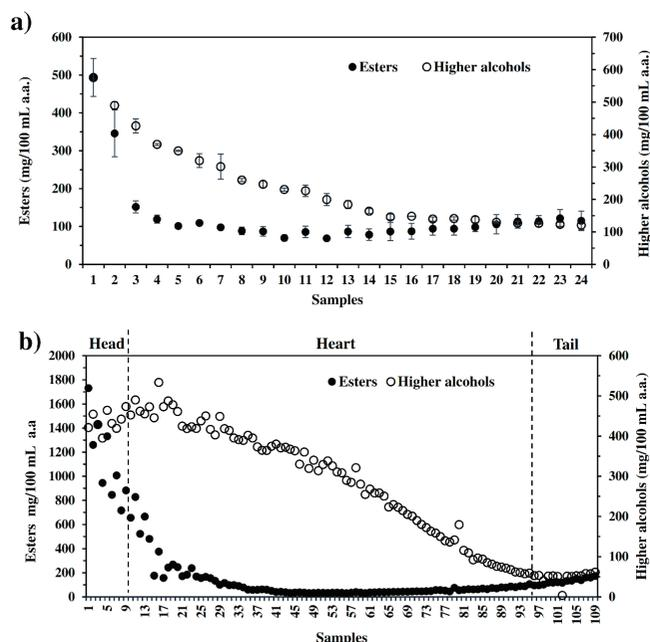
**Figure 2.** Behavior of higher alcohols and esters during the first (a) and second (b) distillation of artisanal Mezcal. The vertical dotted lines on figure "b" indicate the distillate cuts. In figure "a", concentration values are given as the mean of the samples from two copper stills  $\pm$  standard deviation.
