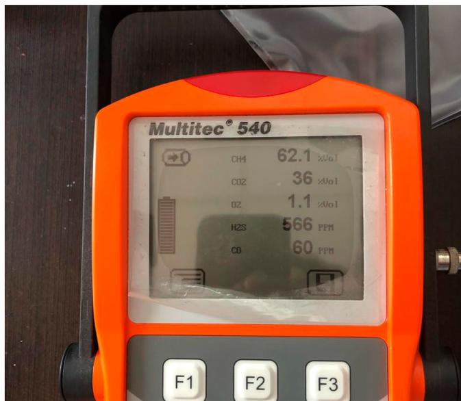
**Figure 2.** Multitec<sup>®</sup> 540 equipment used for the characterization of biogas from each of the experimental trials with the mixture of cattle manure and cheese whey.
