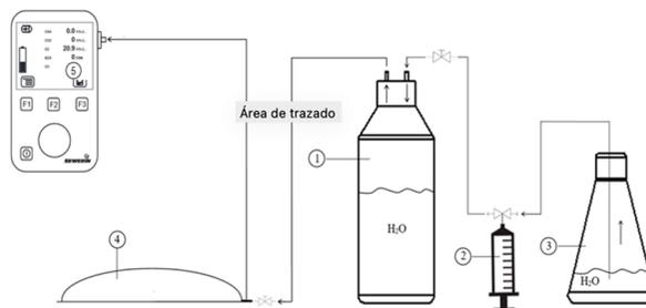
1. Adapted flask (1 L) 3. Collection conical flask (1 L) 5. SEWERIN MultiTech 540 quantizer
