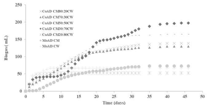
**Figure 4.** Kinetics biogas yield accumulated in the different treatments in mono-digestion (MoDA) and co-digestion (CoDA) in batch tests.
