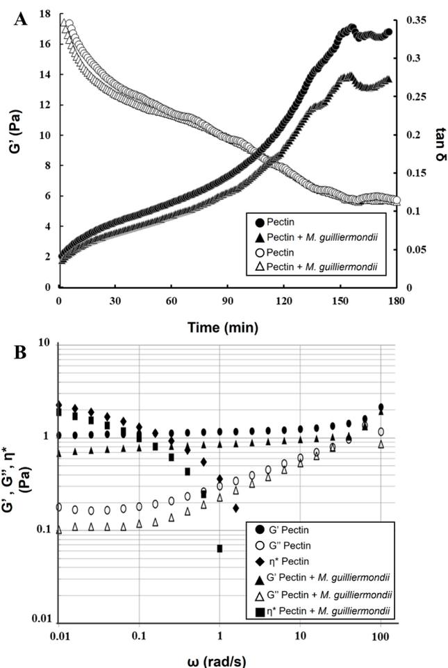
**Figure 2.** Gelation kinetics (A) on film-forming dispersions of pectin and pectin + *M. guilliermondii* and damping material values ( $\tan \delta$ ) vs film-forming dispersions time at 25 °C and 1 rad/s, and frequency sweep (B) on film-forming dispersions of pectin and pectin + *M. guilliermondii* with 1% (w/v) of pectin and 0.5 mM of  $\text{CaCl}_2$  at 25 °C and 1 rad/s.
