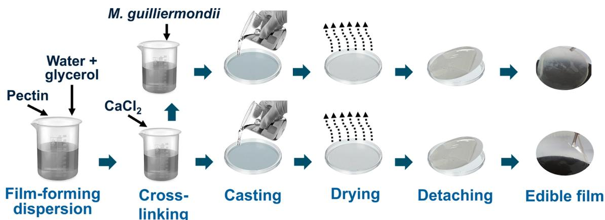
**Figure 1.** Schematic representation of edible films obtention with and without *M. guilliermondii*.
