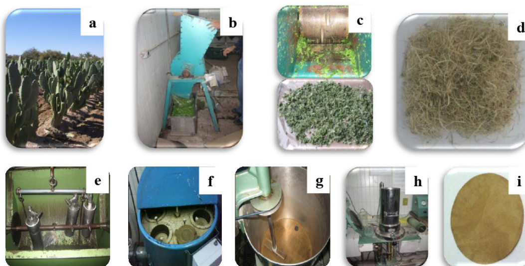
Figure 3. General process of Opuntia ficus-indica pulping. a) Raw material; b) Hammer mill c) Dry raw material; d) Fiber bundles; e) Cooking; f) Beating; g) Screening; h) Paper sheets forming; i) Final paper sheet.
